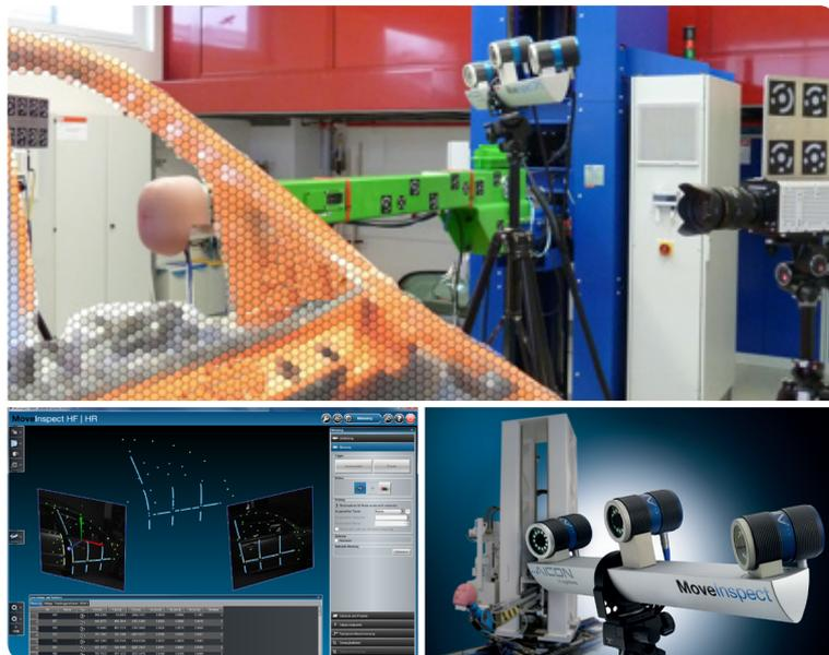
—→ Free Motion Head tests are supported by AICON's measuring system MoveInspect HR and the software module Move 6D
